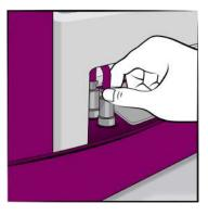
Disconnect the 2 metal connectors for the turntable.
