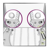
Remove the 4 large hand screws holding the corner light columns.
