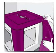
Install and secure the top with 4 large white hand screws. **Note:** If you use the acrylic side diusion panel with the opening, remove the side wall and attach the reflective door cover for convenient side loading.
