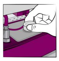
Unscrew the 4 large hand screws holding the built in turntable module.
