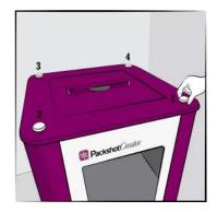
Secure the top using 4 large white hand screws.
