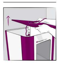
The Packshot*Start* 360 can be entirely dissembled for easy storage or transportation. Remove the 4 white hand screws and take off the top.
