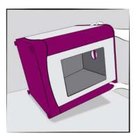
**Note:** Remove the acrylic and glass turntable platforms and tape the driving module down to secure before you proceed to lay the studio down.
