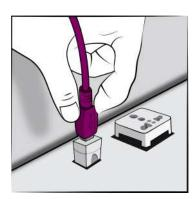
Connect the other end of the USB cable into the USB port located inside the studio.
