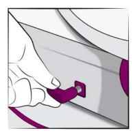
Plug one end of the power cable into the turntable.
