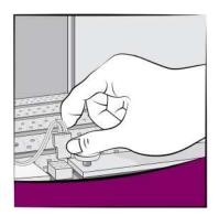
Disconnect the cable connecting the bottom light with the base.
