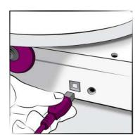
Plug one end of the USB cable into the turntable.
