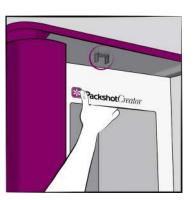
Replace the top. Make sure to orient the top so that the camera strap goes le to right when viewed from the front. **Note:** Align the acrylic panels with the holding brackets at the top to hold them in place.
