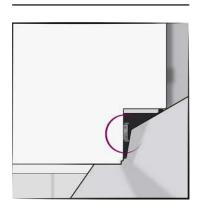
Be sure to place the panels on the holding brackets at the base.
