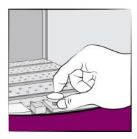
Remove the white hand screws on each side of the bottom light.
