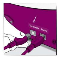
To complete USB connection, plug one end of another USB cable into the left side of the light box ("Turntable port").
