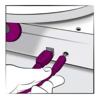
(**Optional**): If necessary, the custom shutter release cable from the camera can be connected to either the system or the turntable so software can automate 360 degree image capture.
