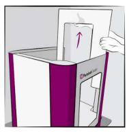
Remove the acrylic side diffusion panels and both side walls.
