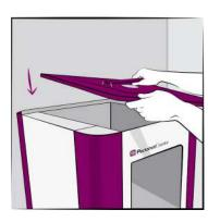
Replace the side walls and top then secure the four white hand screws.
