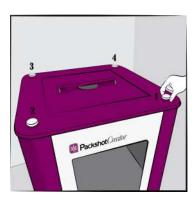
Remove the four white hand screws and take off the top.
