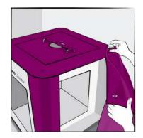
Fix the top using 4 white hand screws. If you use the acrylic side diffusion panel with the opening, remove the side wall and attach the reflective door cover for convenient side loading.
