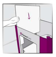
Three acrylic side diffusion panels came with the system – two solid and one with an opening. Choose which two panels to use. Slide in the panels from the top.
